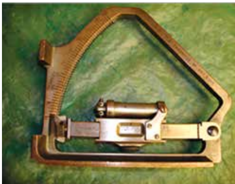
Sydney Baker's Clinometer Filed Mark III No. 6913, Circa 1915 Mfr. CSI Co. Ltd. Cambridge.
